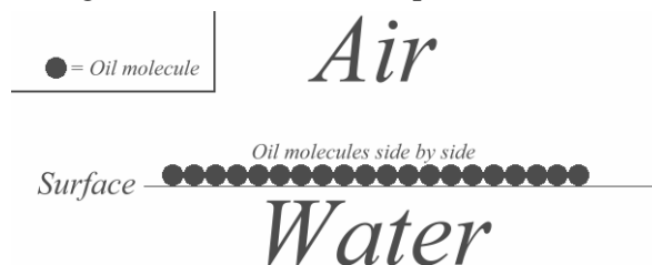
Figure 4.1 How certain oils spread on the surface of water. Although the molecules are shown as round, they are really elongated, with one end that is attracted to the water surface, and another end that is repelled by it.
